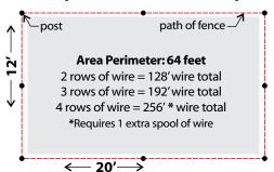
A simple dimensioned sketch can help you determine fence post and fence wire quantities.
